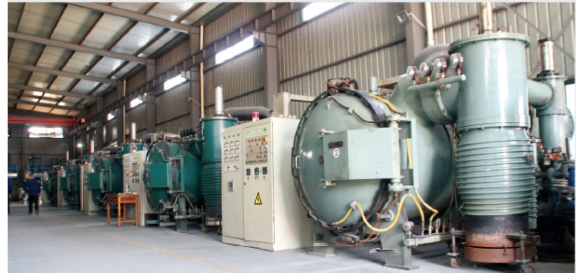
5. 真空烧结 Vacuum Sintering
