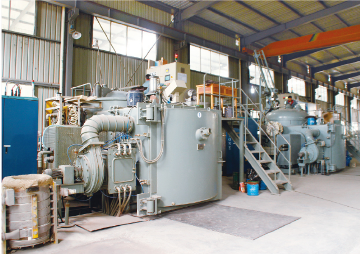
1. 真空熔炼 Vacuum Smelting
